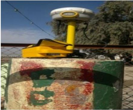
**Fig. 5.** GNSS installation on control point (P4),(field work)
