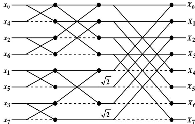
Figure.(3). Signal flow graph of 8-point improved radix-2 FHT algorithmsolid and dot lines stand for addition and subtraction respectively
