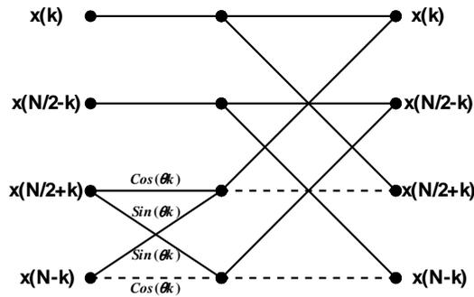
Figure. (1) An in-place butterfly structure of the radix-2 DHT, where  $\theta = 2\pi/N$ , solid and dotted lines stand for additions and subtraction respectively.
