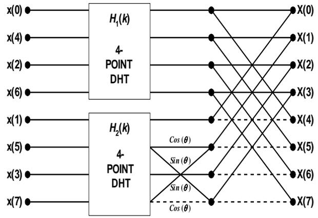
Figure. (2) Construction of an eight-point DHT from two four-point DHTs, where solid and dotted lines stand for additions and subtraction respectively.
