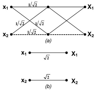
Figure.(4) Partial signal flow graph for the (a) DHT algorithm and (b) Improved DHT algorithm.
