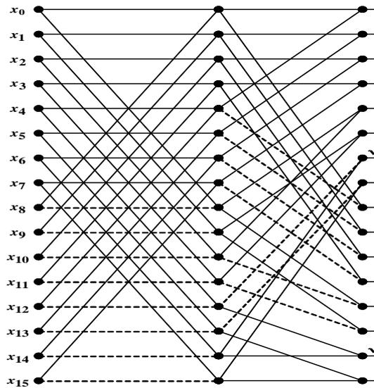
Figure.(5) Signal flow graph of 16-point improved radix-4 FFT algorithm solid and dot lines stand for addition and subtraction respectively
