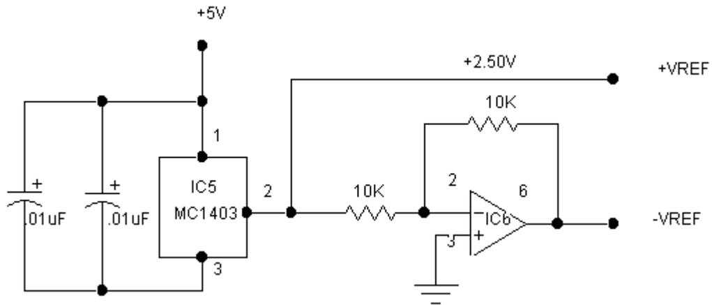
Figure (4-b) Production of 2.50 v source For use with the transmitter in fig 2-a
