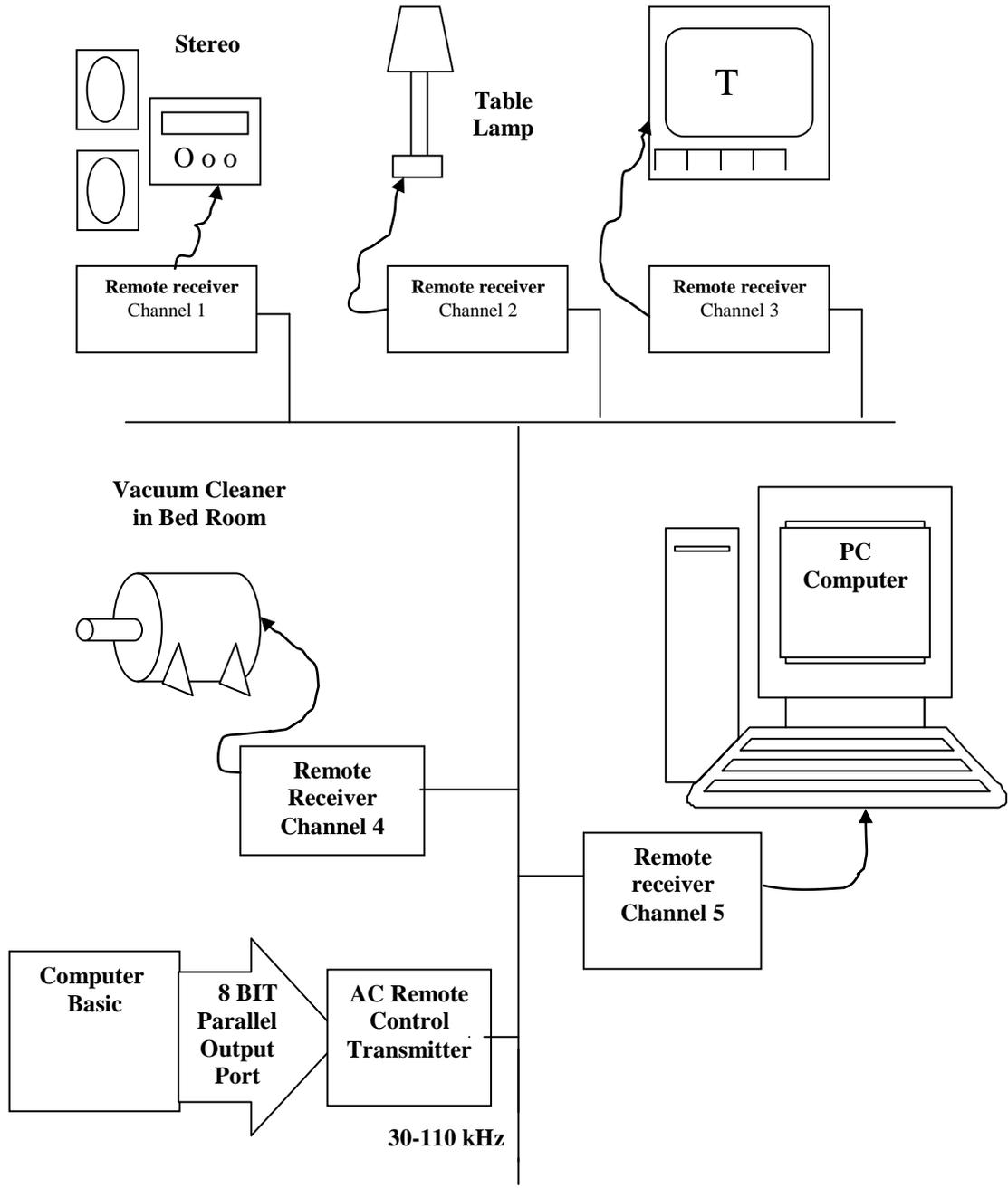
Figure (1): Block diagram of wireless AC remote control system.
