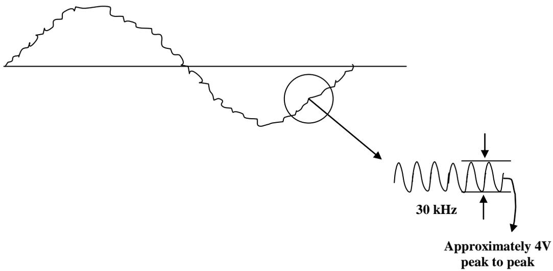
**Figure (3): Example of current transmission**
