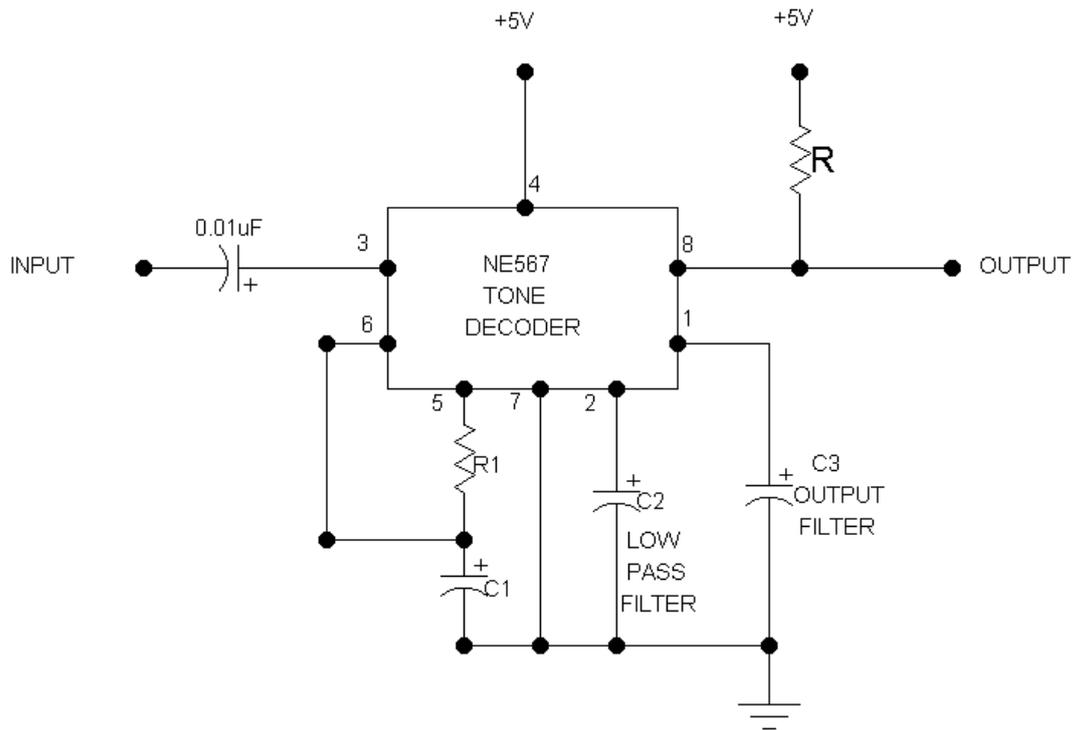
Figure(7) Selection of components for the tone decoder
