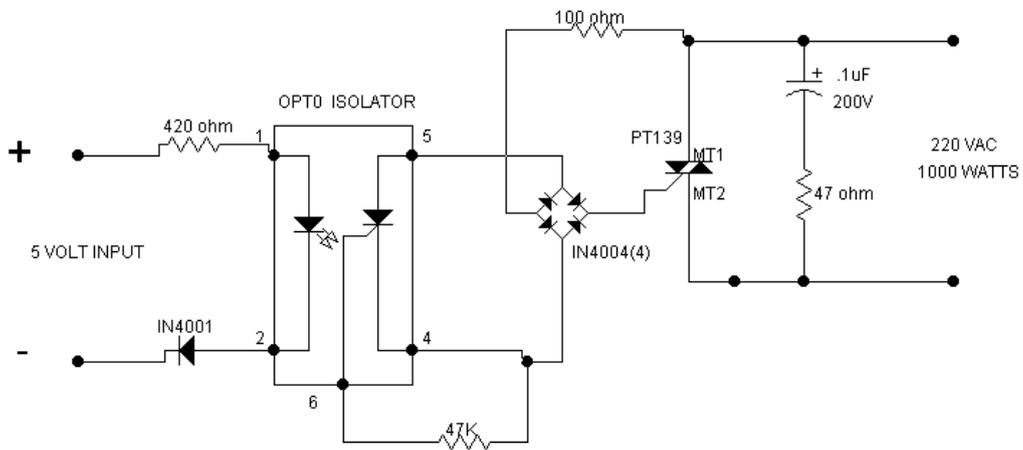
Figure-8: 10A Solid state relay suitable for use in a TTL to 220 VAC application
