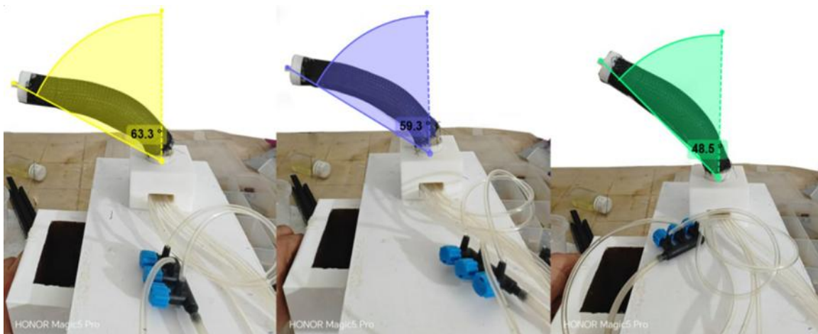
Fig. 6 Bending Angle Values for Three Different Chamber Size Models of the Pneumatic Actuator.
