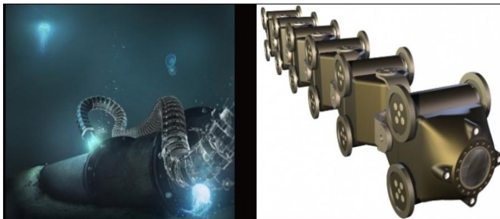
(h) Pipeline Inspection Using a Snake Robot.
