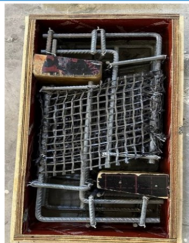
Fig. 7 Preparation of Molds and Reinforcement Placed in the Molds of the Shear Key Specimens.
