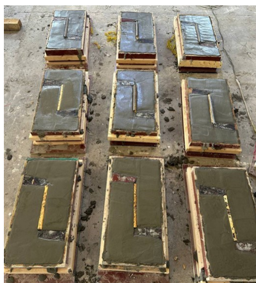
Fig. 9 Making a Groove in Specimens after Refining the Top Face.
