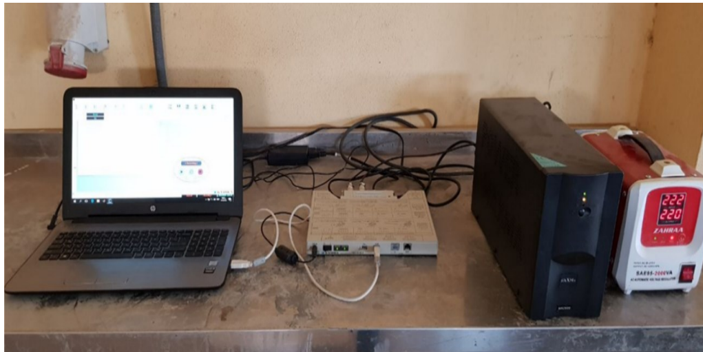
Fig. 12 Load and Deflection Monitoring by the Data Logger.
