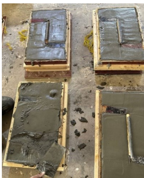
Fig. 8 Casting, Vibrator for Compact, and Finished the Surface by Hand Steel Trowel of the Shear Key Specimens.
