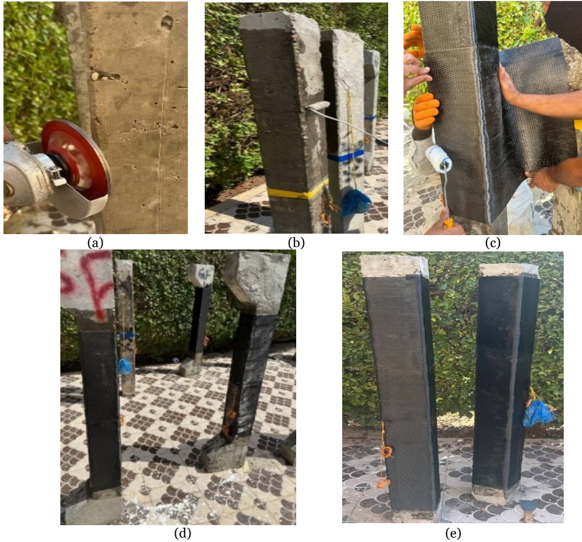
Fig. 7 Strengthening R.C. Columns Specimens [a] Preparation of the Surface and Rounded the Corner, [b] Application of Primer (Quickmast CW ) and Epoxy Adhesive (Quickmast ER 350 ), [c] Placement of One Layer CFRP Sheets, [d] R.C. Column Specimens (CF-C) after Strengthening, [e] R.C. Column Specimens (CF-N) after Strengthening.
