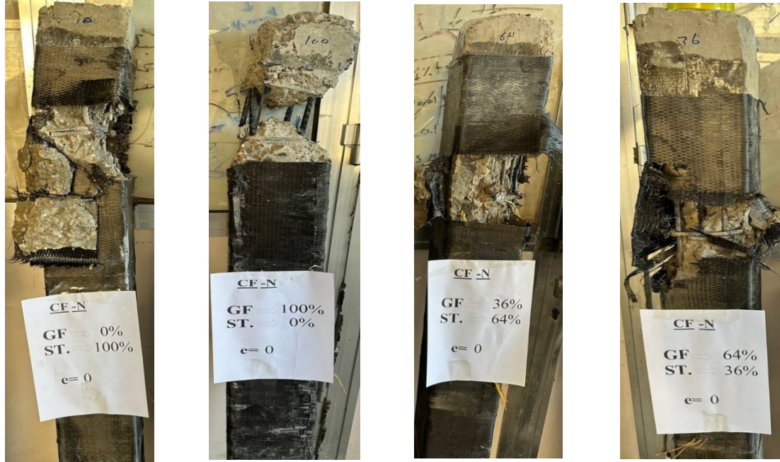
Fig. 10 Failure Modes for Strengthening R. C. Columns Specimens with Eccentricity Ratio e/h=0 .
