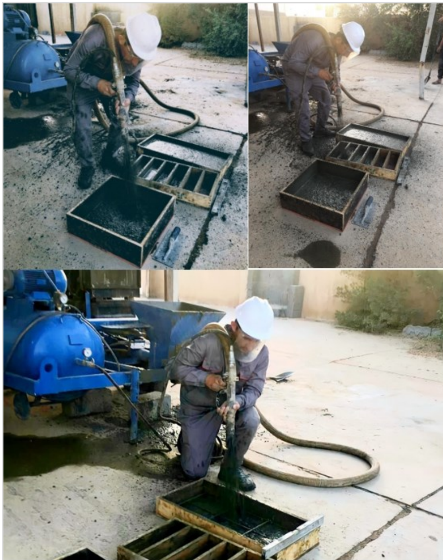
Fig. 6 Casting with Wet-Shotcrete Process: A-Casting Concrete Panel for Compression Test, (B) Casting of Concrete Prisms for Flexural Test, and (C) Casting One-Way Slab Specimens.
