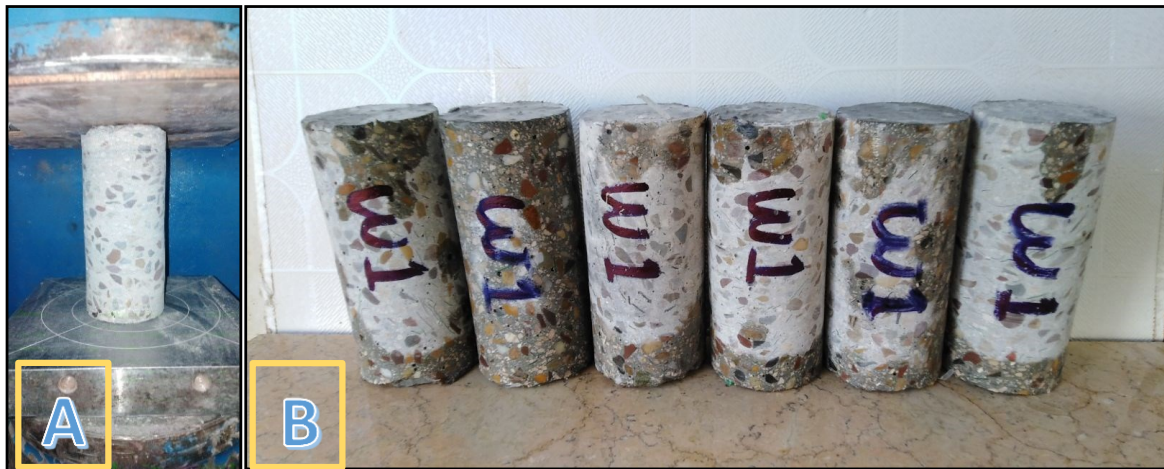
Fig. 8 (A) Compressive Testing of Specimens, (B) Core Samples.
