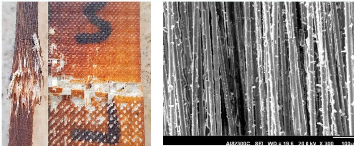
Fig. 3 The GFRP Laminates at Exposure to T_g Temperature and Images of the SEM Test.
