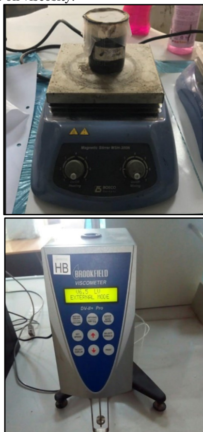
Fig. 1 The Magnetic Stirrer and the Viscometer of Type Brookfield Used in the Experiments.
