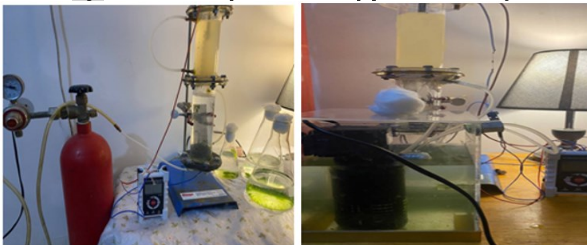
Fig. 2 Microbial Carbon Capture Cell while Operating Both in an Open-Closed Circuit.
