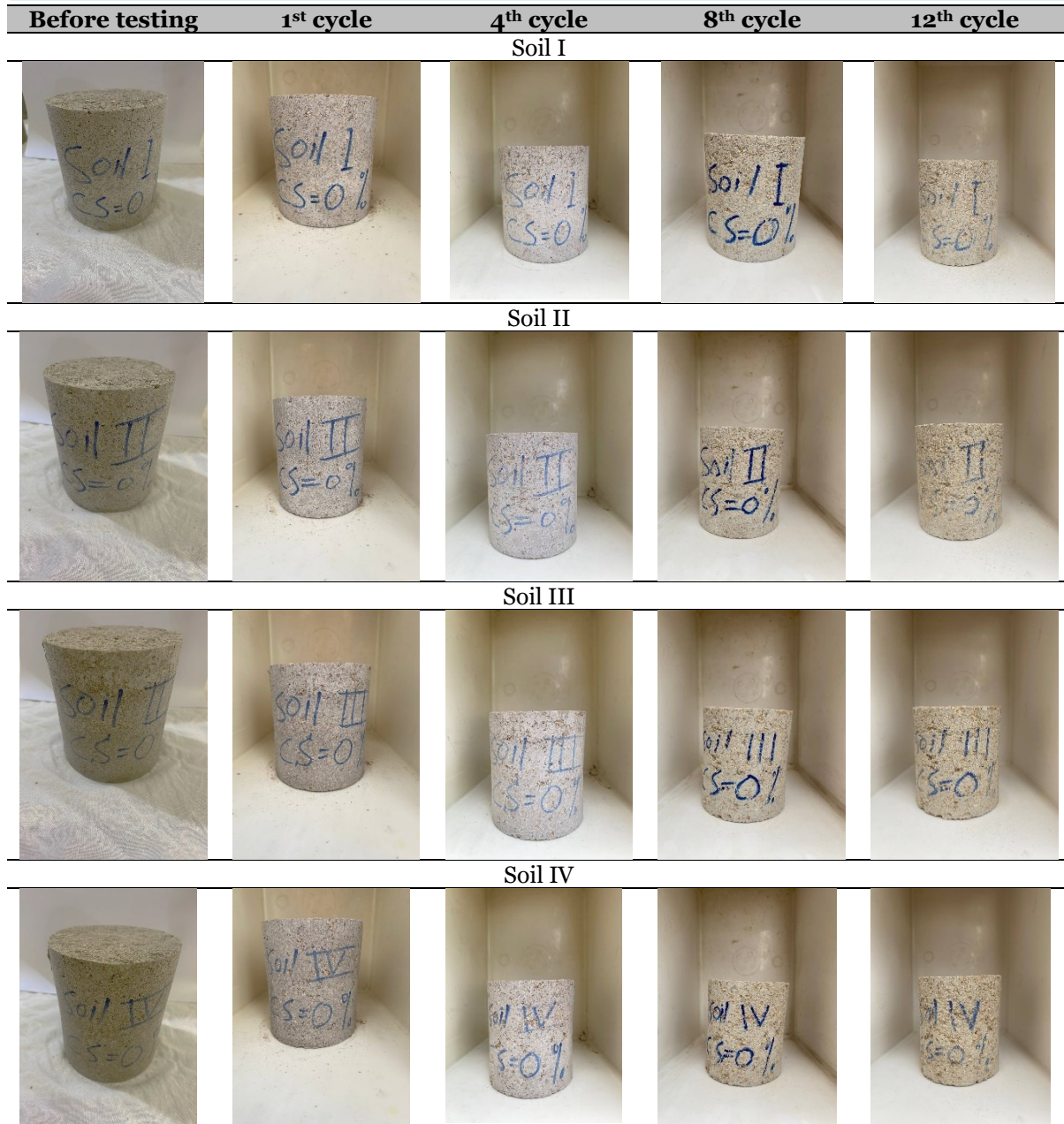
Fig. 18 Wetting-Drying Durability Test Performance for the Soils Treated with 10% Cement.
