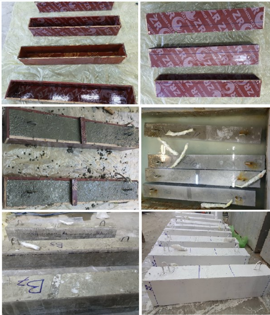
Fig. 1 Preparing Molds, Casting, Curing and Coloring the Specimens.
