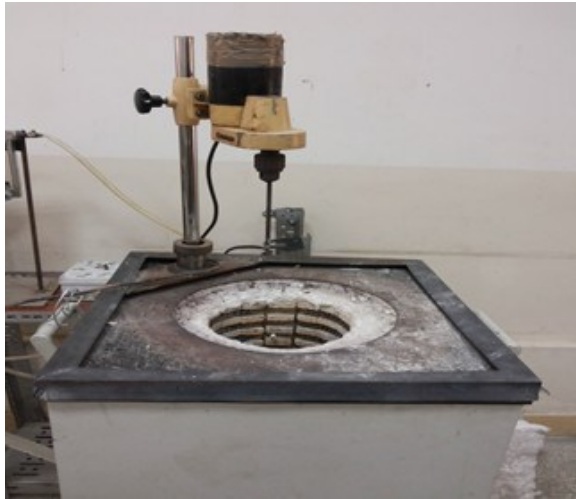
Fig. 3 Stir Casting Method.
