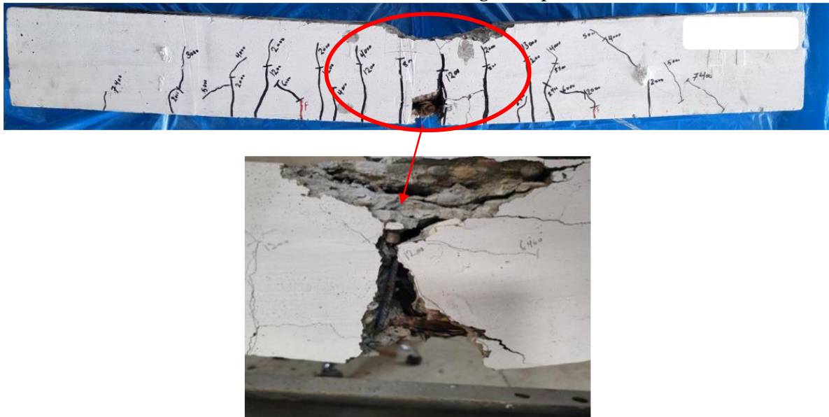
Fig. 5 GFRP Bars Reached a Temperature of 300 °C in Beam (BT4.90).
