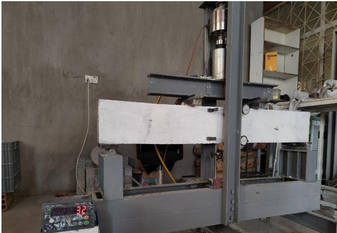
Fig. 3 The GFRP-RC Beam Specimen Test Setup Following Fire Exposure.
