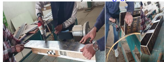
Fig. 3 Preparing the Beam Molds.
