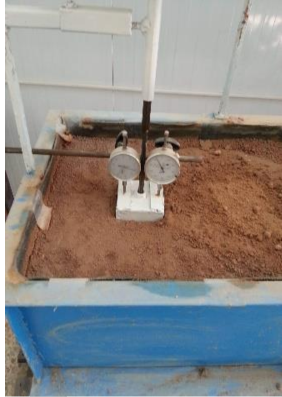
Fig. 5 End of the Square Footing Test.
