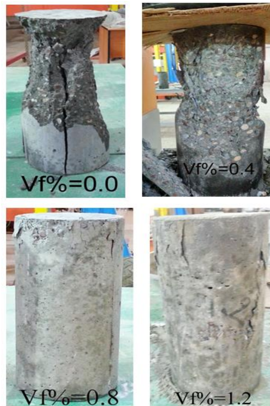
Fig. 11. Typical failed specimens, compression specimen
