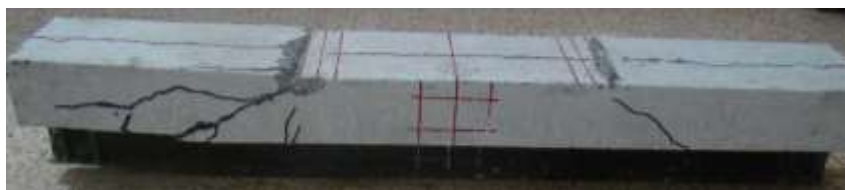
Figure (7) Failure Shape of Tested Beams Sample
