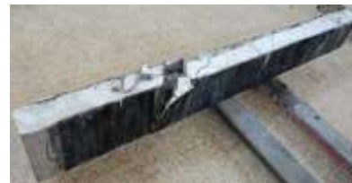
Figure (11). Crack pattern at failure for beam B4.
