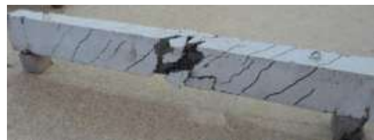
Figure(5) Crack pattern at failure for unstrengthened beam B1.
