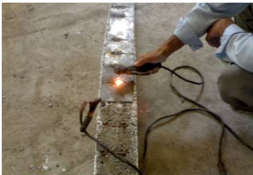
Figure.(3) Making grooves in the tension face of the beam by removing
