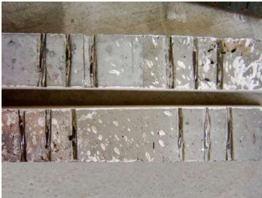
Figure.(3) Making grooves in the tension face of the beam by removing
