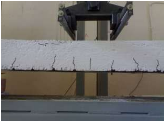
Figure. (13) View of Cracking of Beam B7 (50% Preloading, debonding in two welding point)
