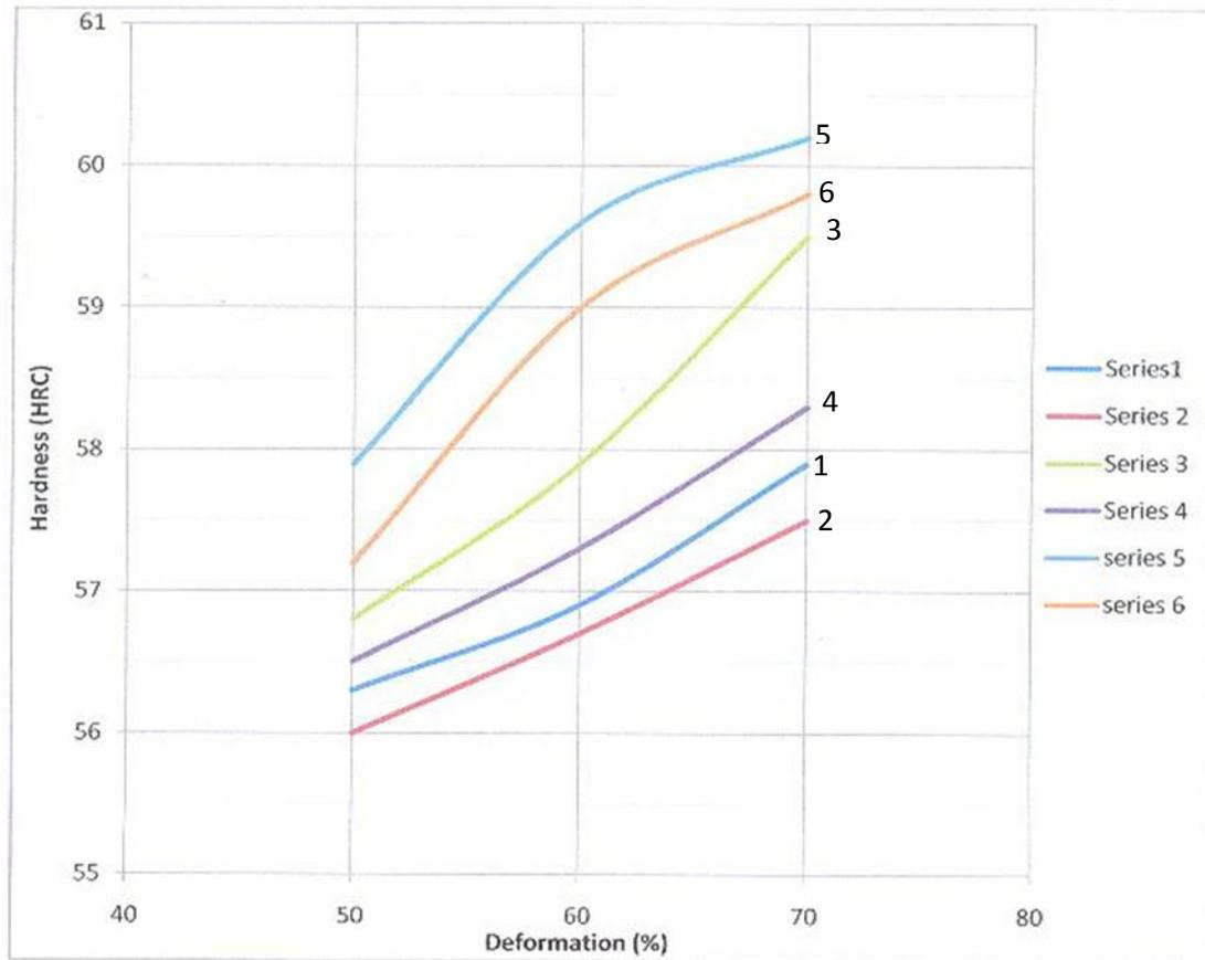
**Figure(3):- Effect the amount of deformation on hardness .**
