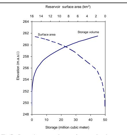
Fig.(5) : Reservoir storage volume surface area elevation curves
